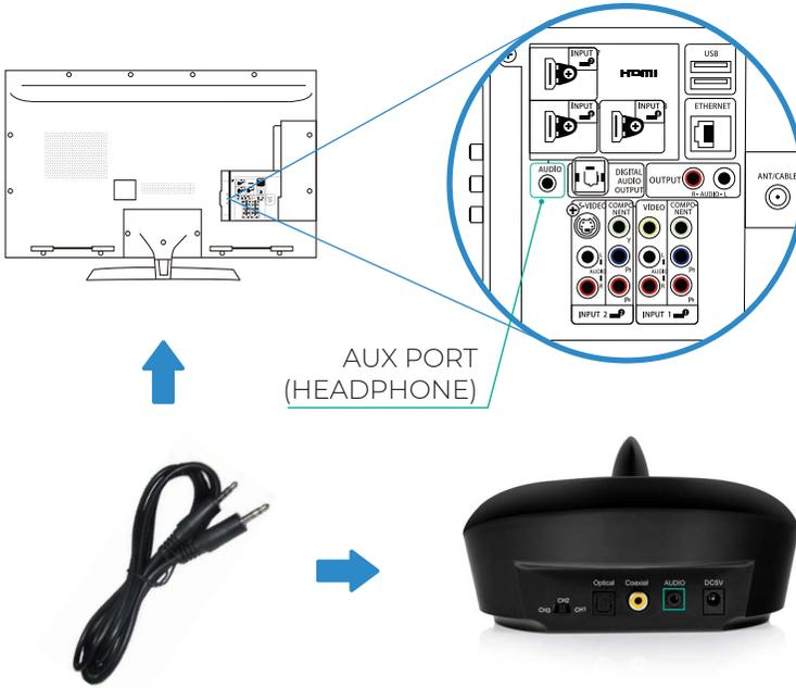
Plug one end of the AUX cable into the TV's AUX Port. Plug the other end into the AUX Port on the back of the transmitter. No sound will come through the TV if using AUX. Sound will only come through the headphones. Adjust the volume of your TV if you cannot hear anything coming from the Headphones.
